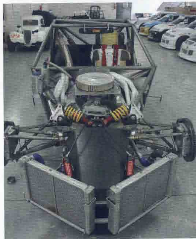
A completely new 4130 steel tube chassis was adopted for this season, after consultation with Nicola Scimeca at the Ycom Consultancy in Italy
