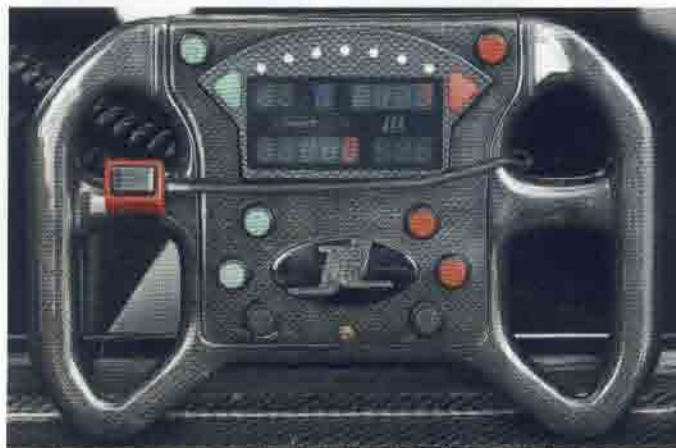
Carbon steering wheel incorporates PI Research data acquisition system
